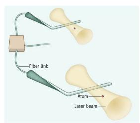
**Toward quantum networks.** Thompson *et al.* trapped atoms with laser beams in the vicinity of photonic waveguide cavities, as shown in the expanded view. The coupling interaction was determined by measuring the emission of photons that escaped the trap through the tip of a tapered optical fiber. These photons, guided by optical fibers, could potentially interact with other trapped atoms. The interactions in these quantum networks could provide a way to store and send quantum information.
